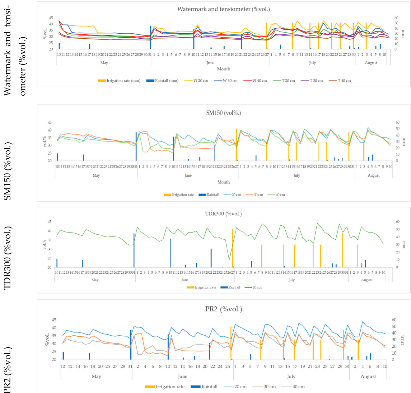
Figure 5. Soil water content (%vol.) monitored with different soil moisture sensors (Watermark, tensiometer, SM150, TDR300 and PR2) at different soil depths (20, 30, and 40 cm).
