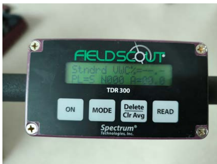
Slika 1. Time domain reflectometry, TDR
